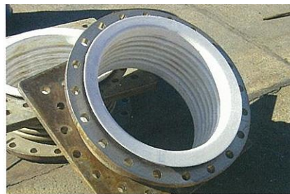
600 NB TEFLON LINED EXPANSION JOINT, USED IN ACID LEACHING PROCESS.
