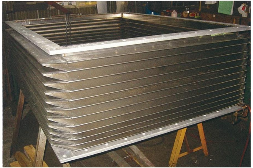
1200 X 1800 RECTANGULAR JOINT USED IN HIGH TEMPERATURE DUCT WORK.
