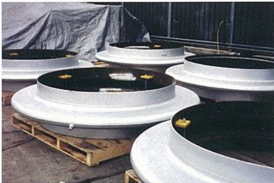
2000 MM DIAMETER HEAVY WALLED EXPANSION JOINT FOR AN ACID PLANT
